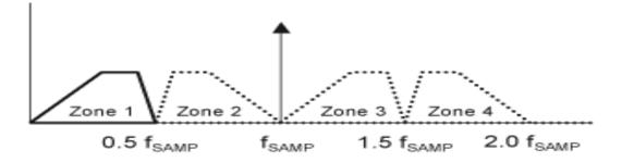
Zone 3 is including the attractive 2m ham radio band and is offering the advantage of no side-band inversion. In the settings of e.g. PowerSDR a 2m DDC/DUC can be easily 'programmed' in the same formal procedure as an analog transverter:
